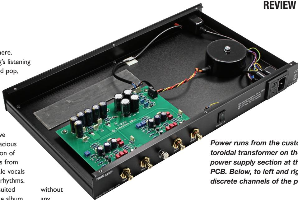
Power runs from the custom wound toroidal transformer on the right, into the power supply section at the top of the PCB. Below, to left and right, are the two discrete channels of the phonostage.
